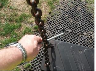
The connecting links are in excess of 8.6mm and less than 12mm and fail the requirements of BS EN 1176 Part 1; clause 4.2.13, Chains Finding:
