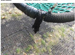
Finding: The rope has worn on the basket Action: Replace rope or net
