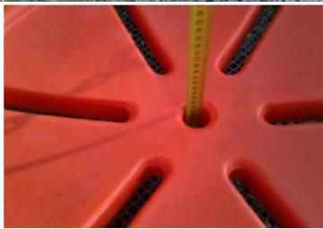
**Finding:** The seat clearance from finished surface level to the underside of the seat is too low when measured in its most onerous position and does not meet the requirements of BS EN 1176 Part 2
